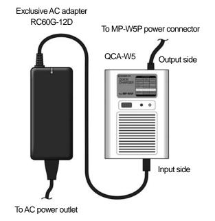
out-of-range. In this case, charging will start automatically as soon as the battery temperature returns to within the battery temperature range. The appropriate charging temperature range is 5 to 35 °C. \* Charging will stop midway if the battery temperature falls out of the
