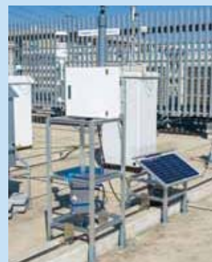
Case with Solar Panel A Solar Panel works as a supplemental power source.
