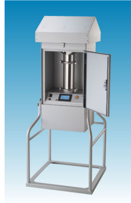
Dioxin Sampler Model: HV-700R Flow rate: 100-700L/min
