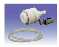
This holder is used for personal samplers and can cut 50% of  $4\mu m$  particles. Inertia colliding method helps to measure personal exposure to the dust during the work.  $4\mu m$  50% cut particles can be collected by sucking the air at 2.5L/min.
