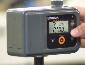
Incorporeates a constant flow rate function to minimize drops. Displaying instaneous and integrated flow volume as digital values. Four timer sampling modes (manual, down, volume, cycle timer). The LCD display for checking in dark locations.
